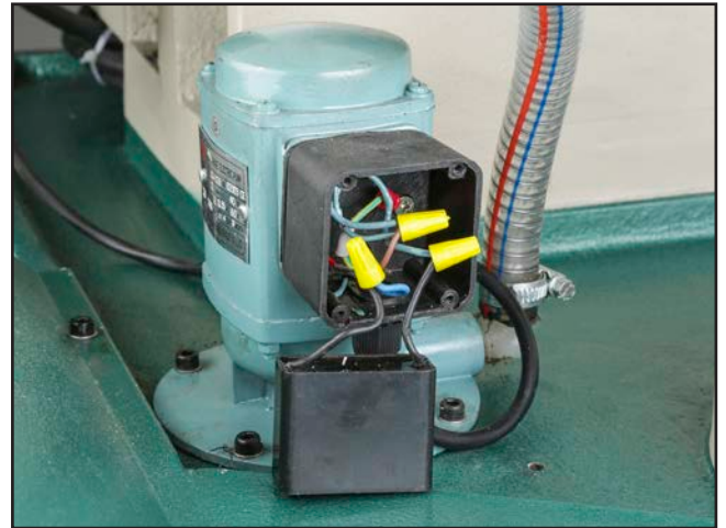
Figure 87. Coolant pump wiring.
